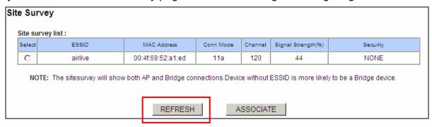
**Step 5** Once the Signal is good enough, please check the radio box in front of the desired AP and then click on the ASSOCIATE button for building the connection.
