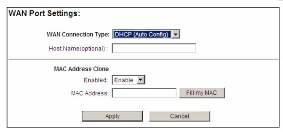
■ Clone MAC Address: Some service provider (Cable Modem provider) lock to certain MAC address. In this situation, the WAN port of AirMax5N needs to clone the MAC address. Please check the "Clone MAC address" box and enter the address that need to be cloned.
