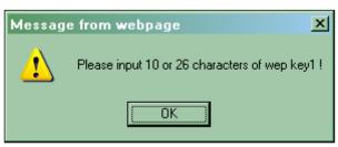
■ **ASCII:** The Key length can be 5 or 13 character to ASCII Key type, and the character can be any ASCII character. If the length is not 5 nor 13, the alert message should pop up as below:
