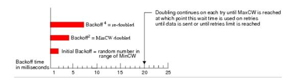
The random backoff used by the access point is a configurable parameter. To describe the random delay, a "Minimum Contention Window" (CWMin) and a "Maximum Contention Window" (CWMax) is defined.
