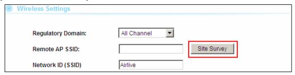
**Step 2** Check the Signal Strength of the desired AP. For identify the AP quicker, we suggest you to written the MAC address of the desired AP and using the MAC to filter out your target.
