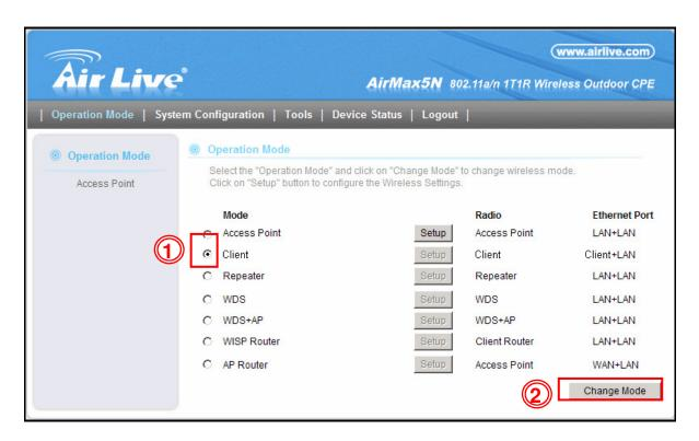
**Step 2** Press "Setup" to enter the wireless settings page. Click on the Site Survey button for searching the remote AP.
