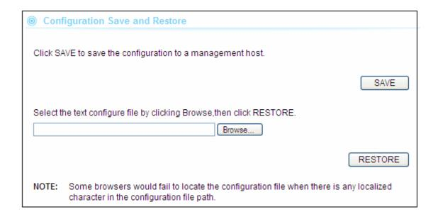
**Step 2** Click the SAVEbutton to save the current configuration into the specified file.
