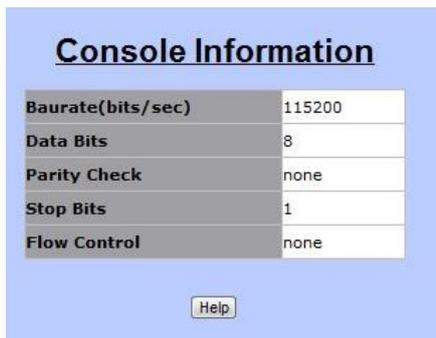
The section is for users to review the settings of console port, which lets users to connect and manage the MINI IP DSLAM in Command Line Interface (CLI) mode.
