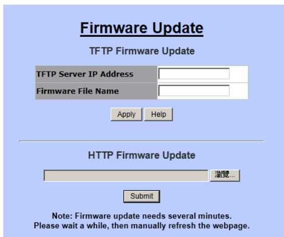
“Firmware Update” allows users to upgrade firmware by themselves. Users are able to choose upgrading firmware through TFTP or HTTP.
