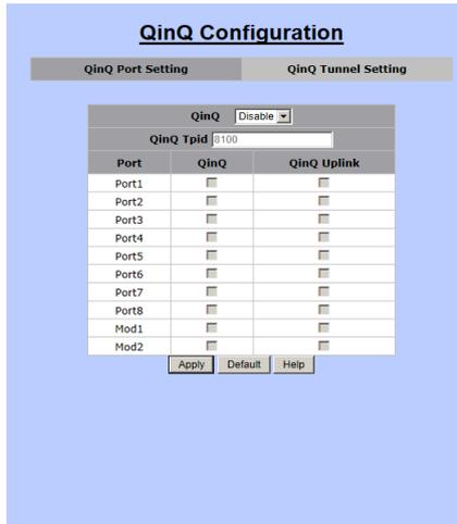
Qinq VLAN function allows users or service providers to separate traffic service for different customers by adding service provide VLAN tags and customer VLAN IDs. In this function, settings are divided into two parts:
