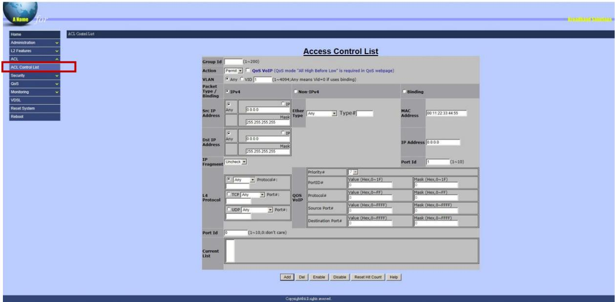
Packets can be forwarded or dropped by ACL rules include IPv4 or non-IPv4. The switch can be used to block packets by maintaining a table of packet fragments indexed by source and destination IP address, protocol, and so on.
