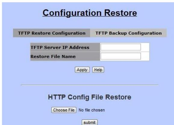
This section is for load the settings from a configuration file. Users are able to upload the settings by TFTP or HTTP.
