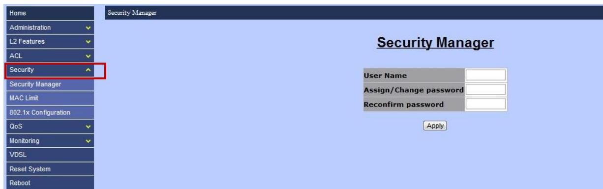
“Security Manager” allows users to change the user name and password for login purpose. Only one set of user name and password is stored in the Switch. The followings are the necessary information for this section.
