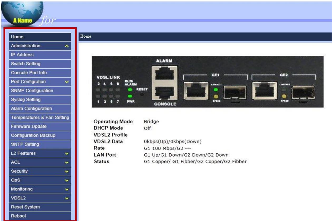
“Menu” section is located on the left hand side of the page and users are allowed to change the configuration and review the status of the device by interacting this section.
