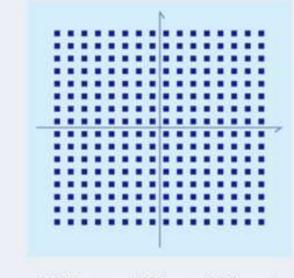
802.11ac: support 256qam modulation mode
