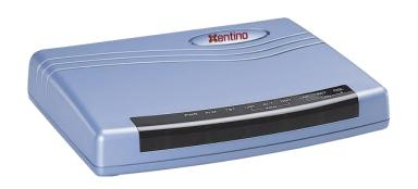
Xentino SR2xx Series 2/4/8-Wire SHDSL.bis EFM Bridges/Routers comply with the latest G.SHDSL.bis technology standards and supports symmetric data rate up to 15.3Mbps/Pair under TC-PAM 128. Up to four pairs can be bonded together for aggregated bandwidth over 61Mbps. It provides a secure and symmetrical high-speed connectivity over existing copper-line infrastructure that is ideal for service providers as well as SOHO and SME users.
