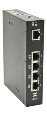
Xentino SI305 PoE series are 5-port (4xGigaPoE + 1xGigaEth), unmanaged full Gigabit Ethernet switches compliant with both IEEE 802.3af and IEEE 802.3at PoE standards and delivering up to 30 watts power per port along with data on standard ethernet cabling. The switches can be used to power IEEE 802.3af/at standard devices (PD), which eliminates the need for additional wiring and ease the deployment for applications to reach power source.
